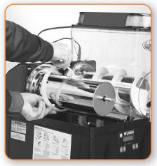
Remove the hopper seal from the flange on the back of the cooling drum.
