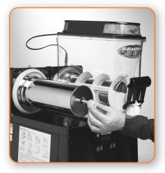
Remove the nose gaskets from the shaft.
