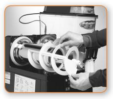
Pull the augers from the cooling drum.
