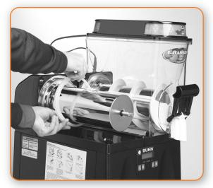
Install the hopper seal over the flange at the rear of the cooling drum as shown.
