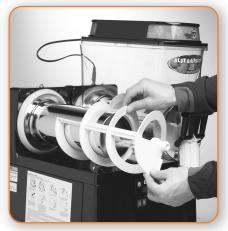
Align the auger shafts with the augers. Push the augers as far as they will go and rotate them so the flat face of the auger shaft is aligned with the flat face of the auger nose.
