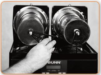
Move shipping bracket to the right and remove from the shaft.
