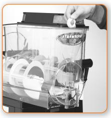
Replace the auger nose bushing inside the front of the hopper as shown in steps 6 and 7.
