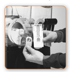
Slide the faucet valve up to remove the spring and faucet seal. Extra care should be taken when handling the seal to prevent damage.
