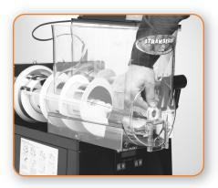
Remove the auger nose bushing from inside the front of the hopper.
