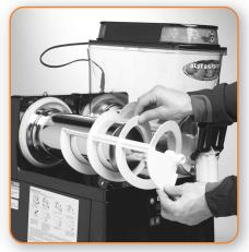
Align the auger shafts with the augers. Push the augers as far as they will go and rotate them so the flat face of the auger shaft is alianed with the flat face of the auger nose.
