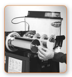
Remove the nose gaskets from the shaft.
