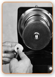
**Spread the lubricant** evenly on the inside of each shaft cone seal with your index finger.
