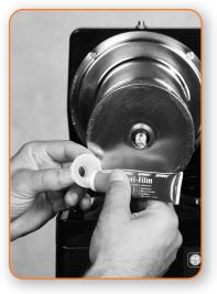
Place a pea sized portion of the food grade lubricant on the inside of each shaft cone seal.
