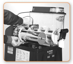
Install the hopper seal over the flange at the rear of the cooling drum as shown.
