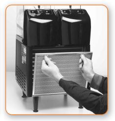
Remove the filter from the rear of the machine and clean thoroughly by running under hot water. Rinse from the inside of the filter out.
