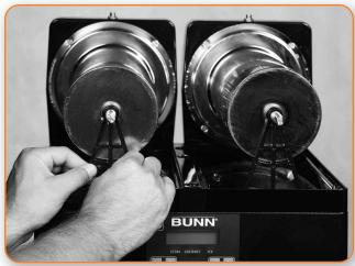
Place hand on shipping bracket and slightly lift up.
