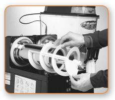
Pull the augers from the cooling drum.
