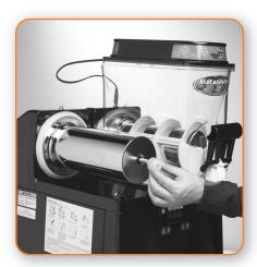
Install the shaft cone seal over the auger shaft with the flat side facing the cooling drum.
