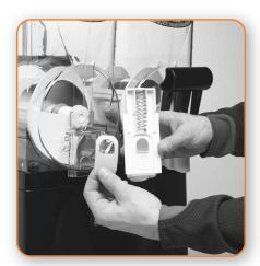
Slide the faucet valve up to remove the spring and faucet seal. Extra care should be taken when handling the seal to prevent damage.
