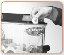
The auger nose bushing is easy to lose, so make sure to KEEP IT IN A SAFE PLACE during cleaning.
