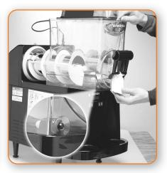
Depress the hopper lock plunger (inset), lift slightly. Pull the hopper assembly forward and remove.
