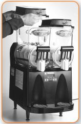
Set each hopper lid on the hopper and plug in each hopper lid lamp cord.
