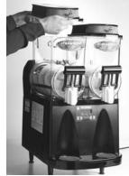
Unplug the hopper lamp cords and remove the hopper lids
