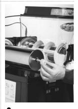
Remove the nose gasket from the shaft
