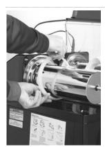
9 Remove the hopper seal from the flange on the cooling drum
