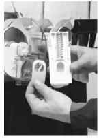
Carefully slide valve up to remove spring and faucet seal. Extra care should be taken when handling the seal to prevent damage
