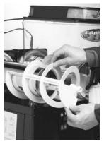
Pull the auger from the cooling drum
