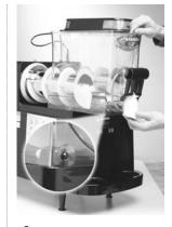
Depress the hopper lock plunger (inset), lift slightly. Pull the hopper assembly forward and remove
