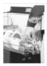
Remove the auger nose bushing from inside the front of the hopper
