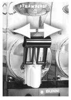
Spread one side of the handle first, then the other and disconnect from the hopper
