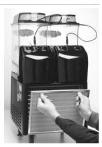
Remove filter from rear of machine and clean thoroughly by running under warm water
